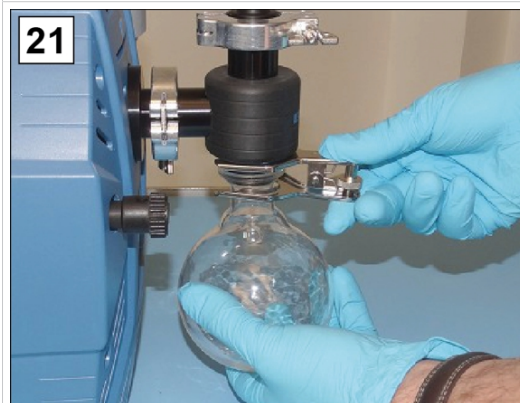
21. Fasten the glass flask to the inlet IN.
