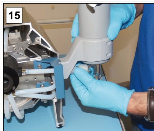
15. Fasten the union nut from the inflow EK.
