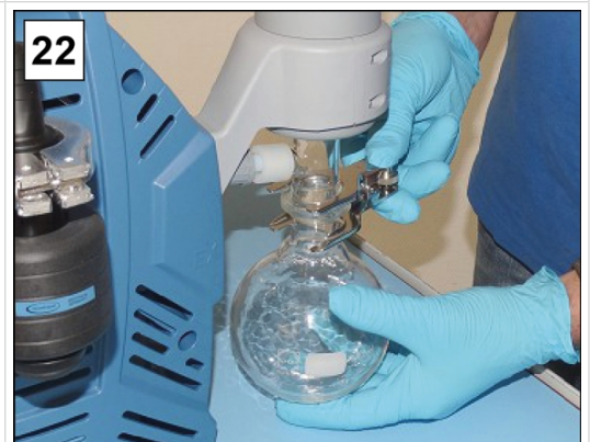
22. Fasten the glass flask to the EK.
