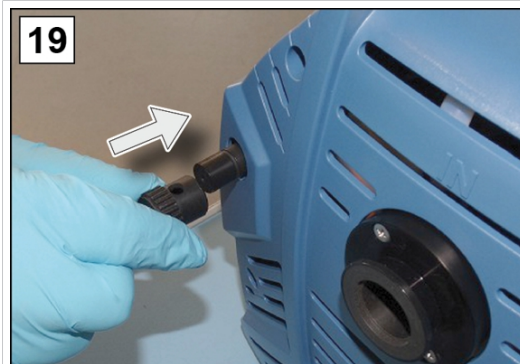
19. Place the cap onto the gas ballast.
