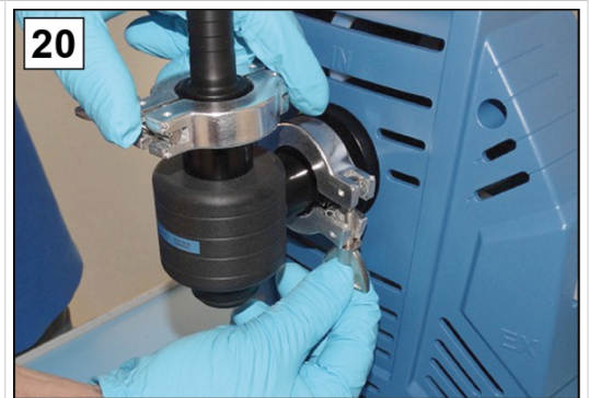
20. Fasten the inlet separator to the tension ring.
