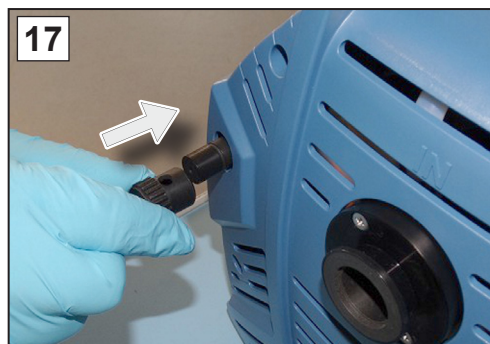
17. Place the cap on the gas ballast.
