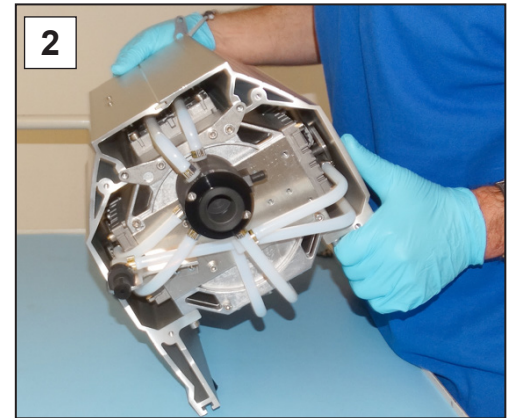
2. Place the pump carefully on its side.
