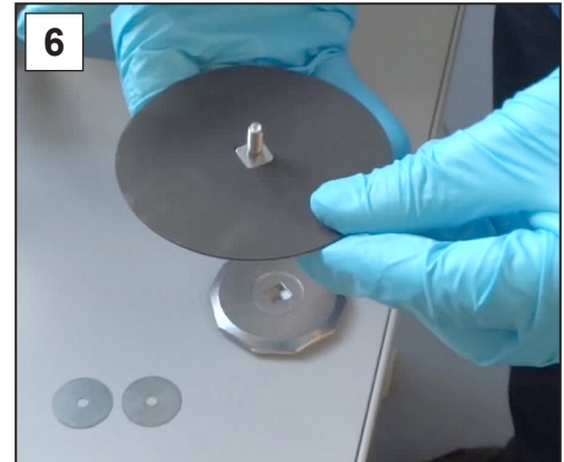
6. Place the new diaphragm over the square head of the clamp- ing disc.
