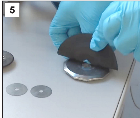
5. Pull out the diaphragm clamp- ing disc and remove the used diaphragm.
