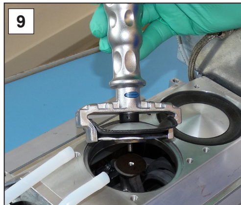
9. Hold the spacer discs firmly and place all the components carefully on the connecting rod thread.
