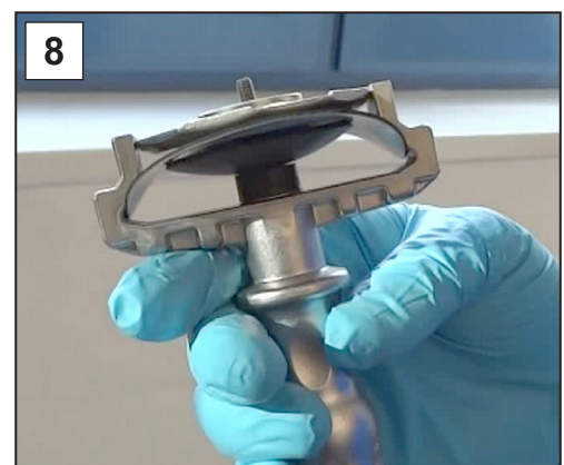
8. Secure the diaphragm assem- bly inside the diaphragm wrench.
