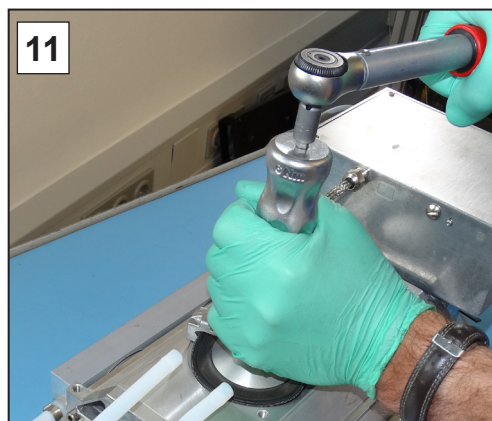
11. Then position a torque wrench with socket head bit on the diaphragm wrench and tighten the assembly to 6 Nm.
