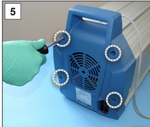
5. Unscrew the 4 screws from the rear housing section; hex key size 4.
