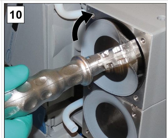
10. Initially tighten the assembly with the diaphragm wrench by hand.
