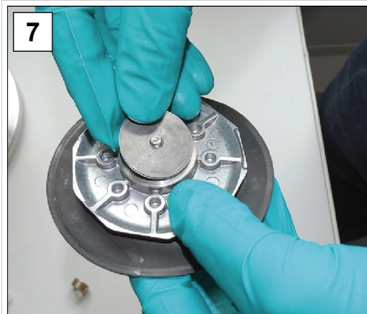
7. Place all spacers onto the threaded bolt.
