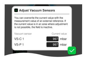
Pop-up for the adjustment of connected vacuum sensors at ambient pressure and under vacuum.
