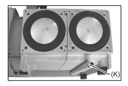
➡ Bring the diaphragms (F) into a position, in which they are in contact with the housing (J) and centered with respect to the bore.
