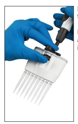
Hold the device over a suitable disposal container and press the ejector to the stop.
