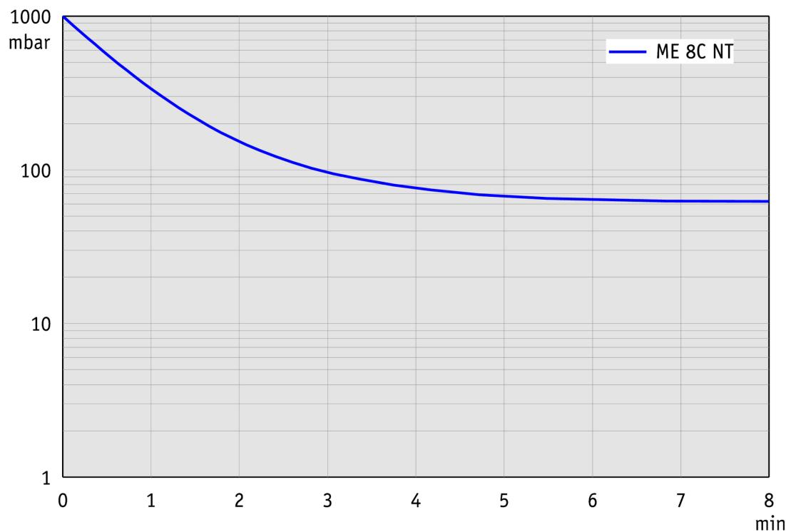
**Courbe de débit à 60 Hz**
