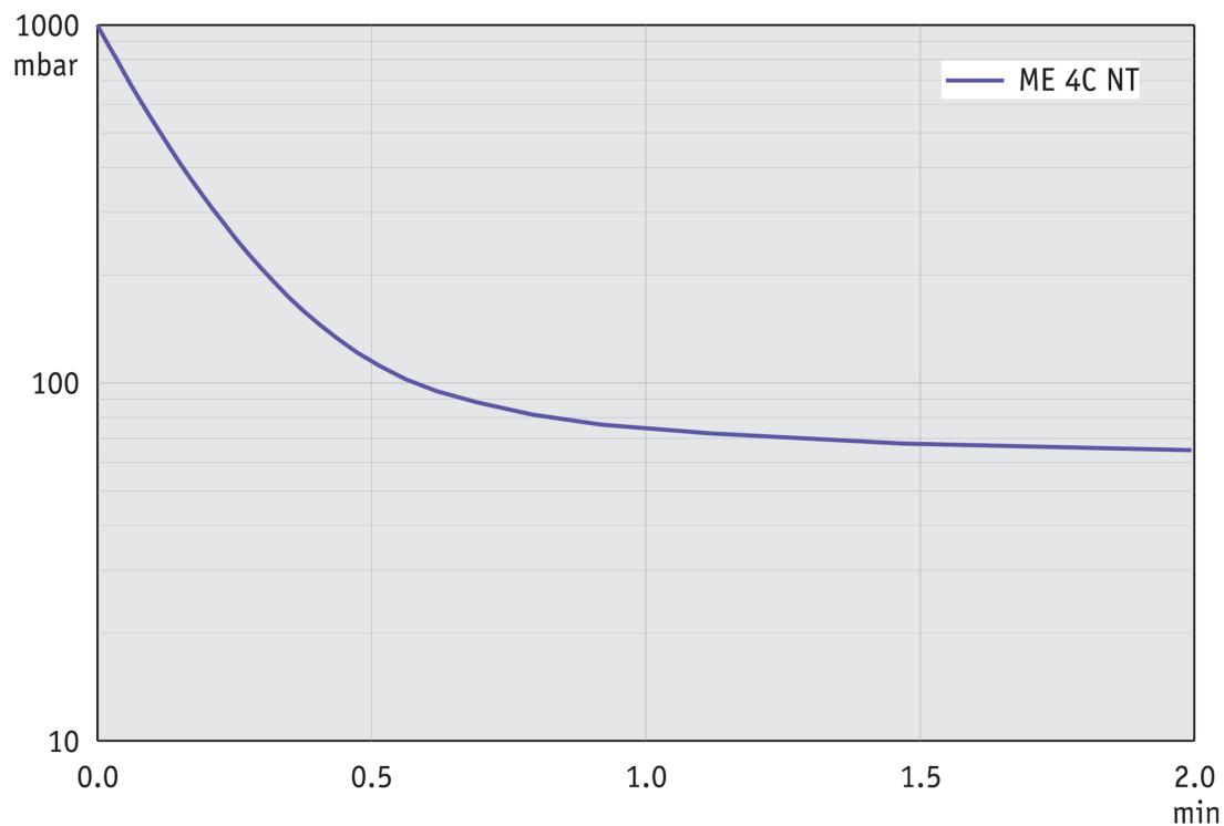
**Saugvermögenskurve bei 60 Hz**
